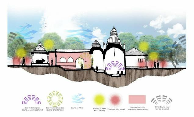
Figure 14: Shukleshwar temple section showing Sound transmission model in temple precinct
